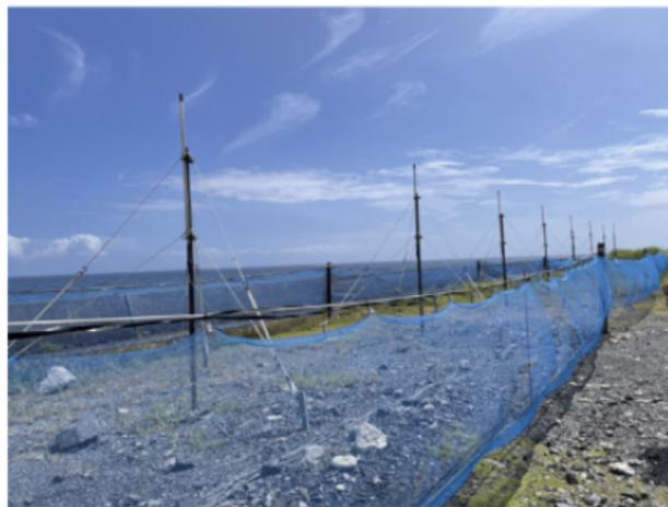
Send the wave spectra with four transmitting array antennas (left side) and receive the reflected wave spectra with eight receiving array antennas (right side). One radar is composed of these transmit and receive antennas. They are placed a few meters from the coast.
